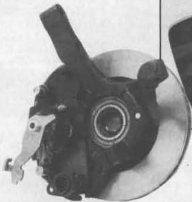
The rear brakes use larger rotors and F-body calipers. The uprights were modified to accept the emergency brake mechanism. The Fiero Pace Car has the braking capacity of a brick wall; you stop right now, no questions asked.
