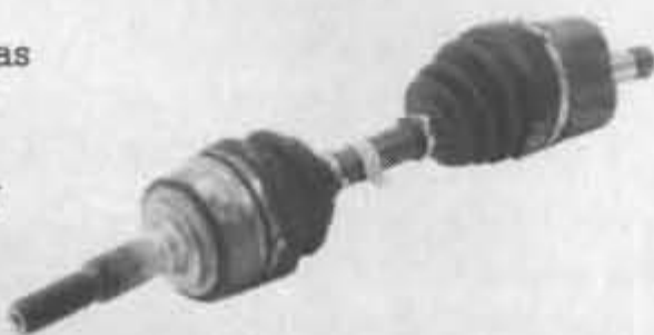
The standard 23mm rear axles were upgraded with HD 27mm axles and hubs from a Pontiac STE. These provided larger bearings to handle high-speed running and allowed the use of larger rotors and Trans Am calipers.
