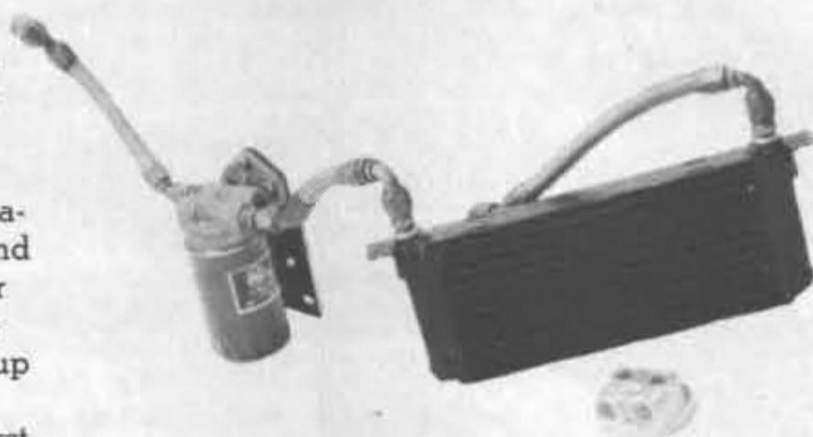
A Rapid Cool oil cooler and remote oil filter system are used to maintain proper oil temperature during high-speed running.
