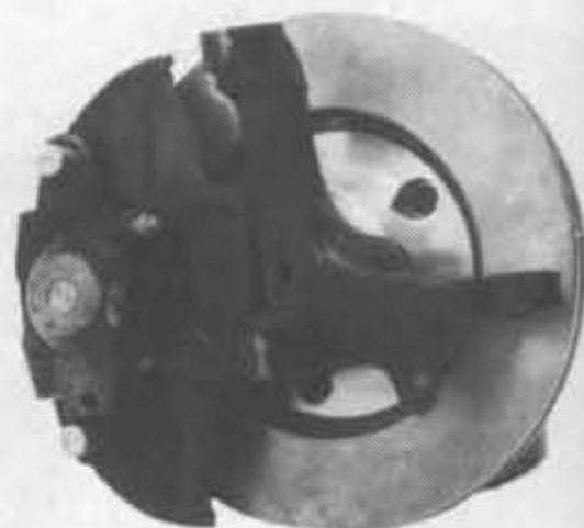
Special aluminum front hubs from Bell Tech Industries, (209) 445-1602, use F-body bearings with a stock Fiero knuckle and Firebird rotors. The assemblies add 28 pounds to the car, but they gain the benefit of larger vented rotors and bigger bearings for outstanding braking with repeatable non-fade performance.
