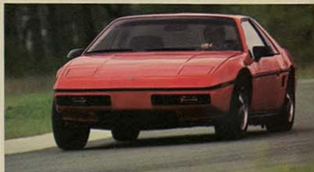
Pontiac's revolutionary building blocks include an X-car powertrain and suspension, a modified T-car front suspension, a unitized steel underbody, and a dozen major molded-plastic body panels.
