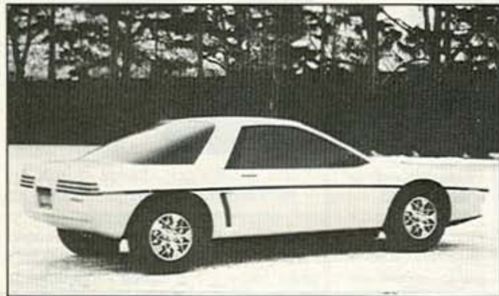
The bubble back (left) was desirable from an aerodynamic standpoint but too expensive. Another Advanced Design study (above) sported windowless B-pillars and a heavy cut line around the car's middle.
