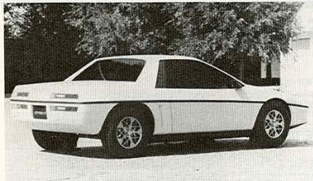
The Advanced III Studio rolled out this revised P-clay model very late in August 1979. Still carrying the Sprint name, this is actually the third version of the original P-car proposal and features a split-lamp rear fascia, vertical lower body air intake, and a window-like trim panel in the C-pillar.
