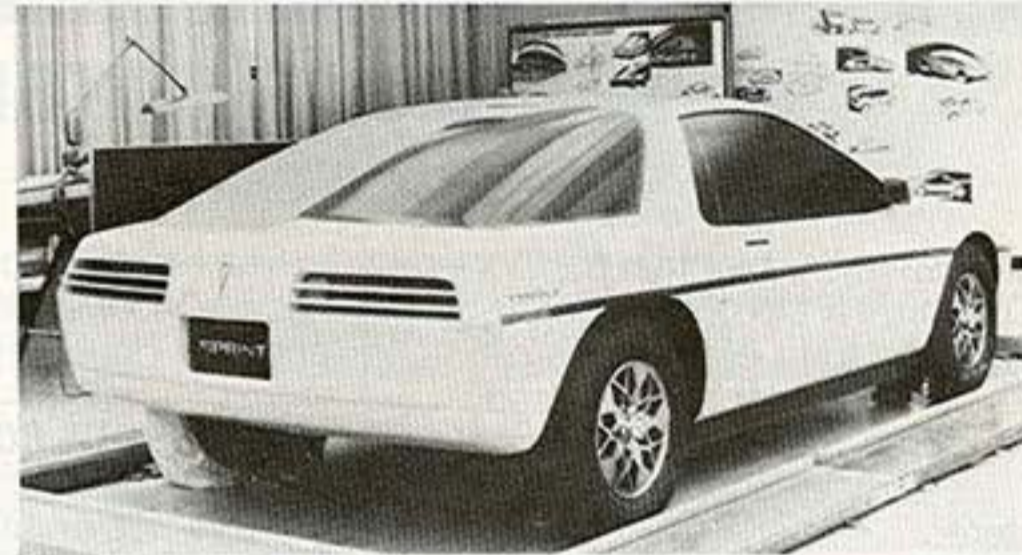
The addition of a bubbleback window and glass quarter window visually changed the first-generation Sprint substantially. The glass quarter window would have to be abandoned since in December 1979, when this model was completed, the P-car's metal substructure was finalized and the near-vertical C-post could not be thinned in time for production.
