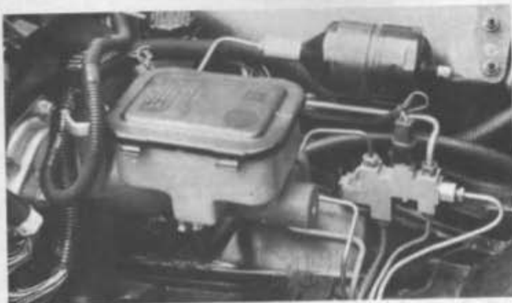
A prototype electrically powered hydraulic master cylinder system provides instant power brakes as soon as the key is turned on. Even with the engine off the car retains full braking capability.
