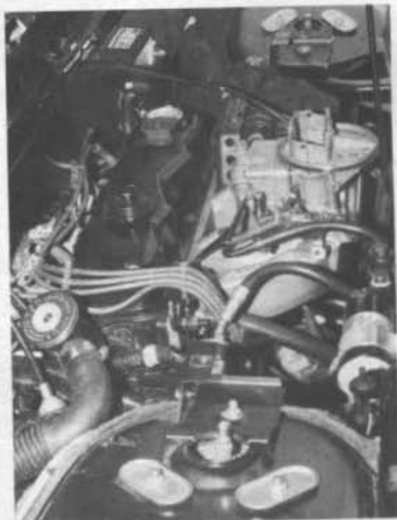
The Super Duty engine pumps out 232 hp with a Holley 2-barrel carb as shown here. For Pace Car duties at Indy, the engine will be fitted with a 115-pound-per-hour throttle body fuel-injection unit with a larger 2 1/4-inch butterfly. The transmission was strengthened with a full gear set from Webster Gears Inc., (415) 388-2728. Webster has a full line of high-strength racing gear ratios for Fiero transmissions.
