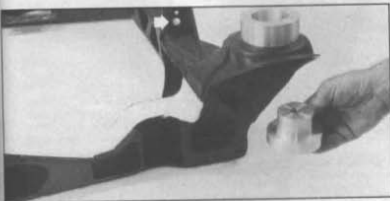
The engine cradle was strengthened top and bottom with .105-inch plate as shown by the white area in the photo. Body mounting hole (arrow) was lowered 5mm to improve torque steer control and mounts were made of solid aluminum. Higher-durometer urethane suspension bushings were also installed.
