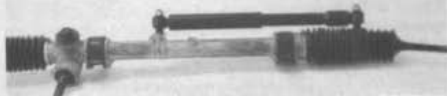
Sweet Manufacturing, (616) 344-2086, makes the necessary internal components to change the production 23:1 steering ratio to 16:1. These are direct replacement parts you can install in the rack on your own Fiero.
