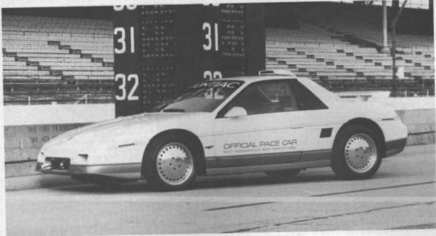
Body modifications for the high-speed Fiero include new aero front and rear fascias, lower side air dams, and rear deck spoiler.
